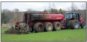
photo illustrates, the corn land has a substantial green crop growing. The piece of equipment is injecting the manure directly into the soil, preventing agricultural runoff. This also provides better utilization of the manure by the corn plants being grown.
